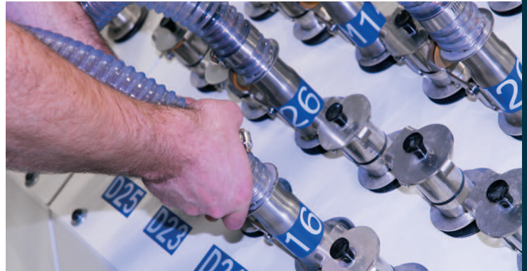
Auto ID proofing option ensures that material moves from correct source to the intended destination.
