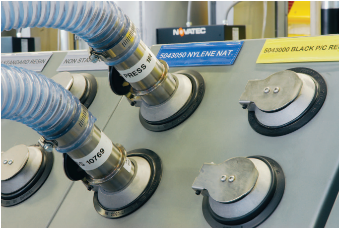
Material and destination names can be clearly marked to help avoid errors.
