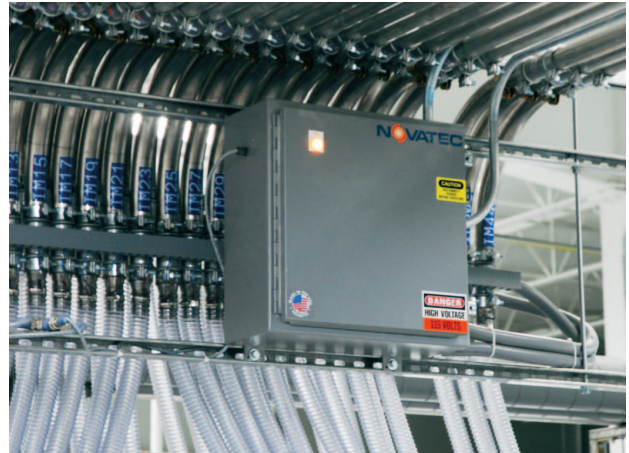
Auto ID Control recognizes any mismatch of source to destination and blocks material transfer.
