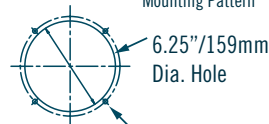
6.25"/159mm Dia. Hole 0.3125"/8 mm Dia. Hole - 4- Equally Spaced On A 6.875"/175 mm Dia. B.C.
