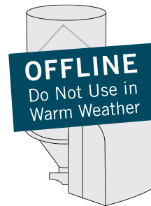
Compressed Air “Dryer” Without Membrane
