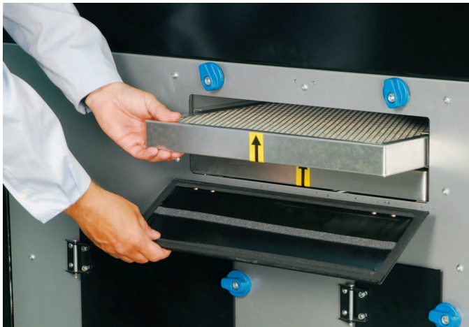
Oversized, dual regeneration blower filters.
