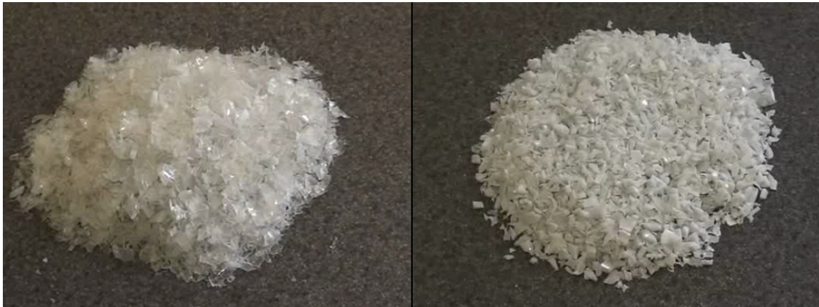
PET sheet regrind is relatively clear before it is crystallized
