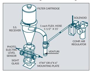
The standard package includes a SS receiver, JIT sight glass, photo electric level sensor, filter cartridge, regulator, venturi, solenoid, 15' of 1-1/2" flex hose and a 1-1/2" aluminum pick-up wand.
