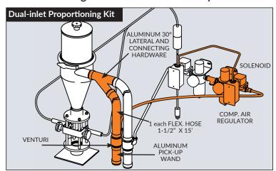
The DIP-1, consists of a  $30^\circ$  aluminum lateral with connecting hardware, an additional regulator, venturi, solenoid, 15' of 1-1/2" flex hose and a 1-1/2" aluminum pick-up wand. (highlighted in orange)
