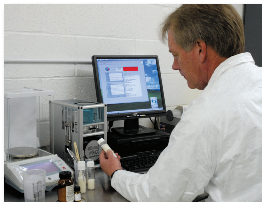
Measuring moisture content of material samples
