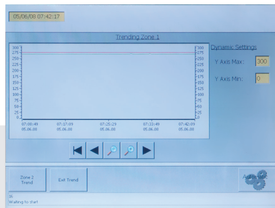
Temperature trending screen for heating zones
