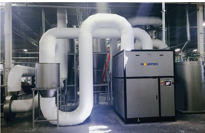
ITPS with Gas-Fired Heater and drying hopper.
