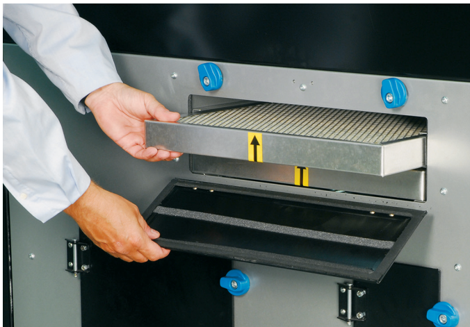
Oversized, dual regeneration blower filters.
