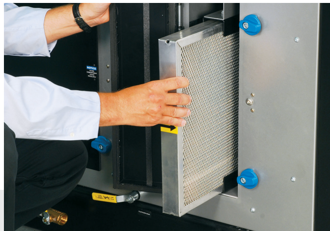
Easily accessed plasticizer filter for cleaning.
