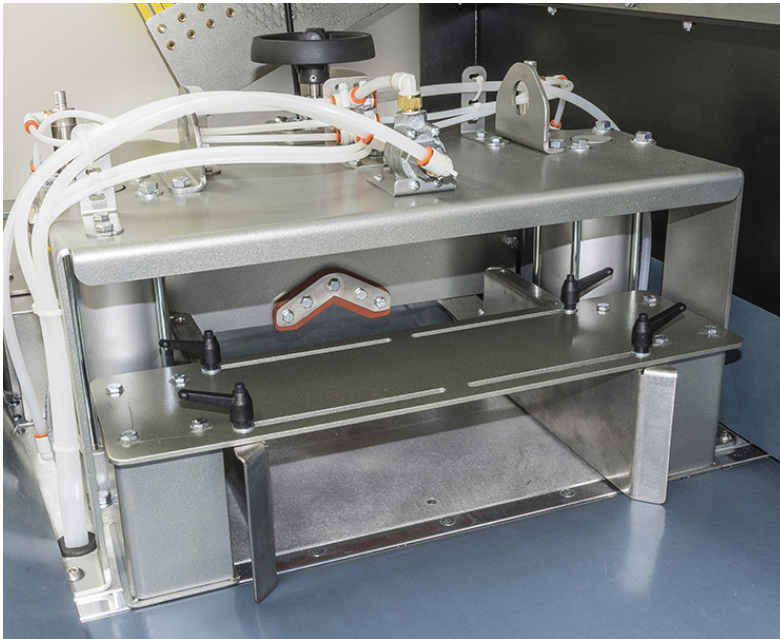
Clamp plate shows manual screw adjustment and quick-adjust product guides.
