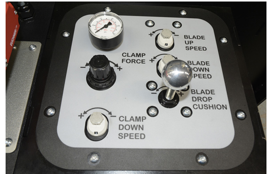
Pressure and speed control for saw blade and clamp motions
