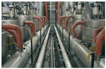
**Closed loop manifold provides** -40° dew point dry air to hoppers and returns moisture laden air to central dryer.
