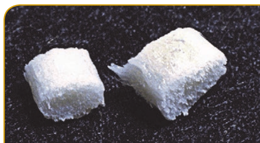
Close up shows sharp edges on glass-filled pellets that damage conveying components.
