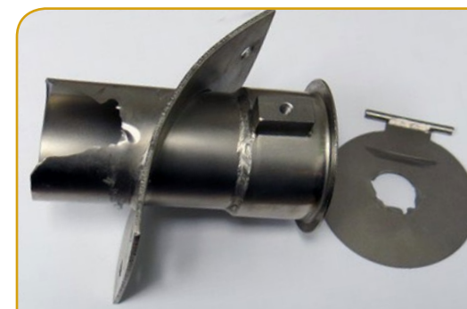
Abrasive Pellets severely damaged this receiver inlet and inlet valve.
