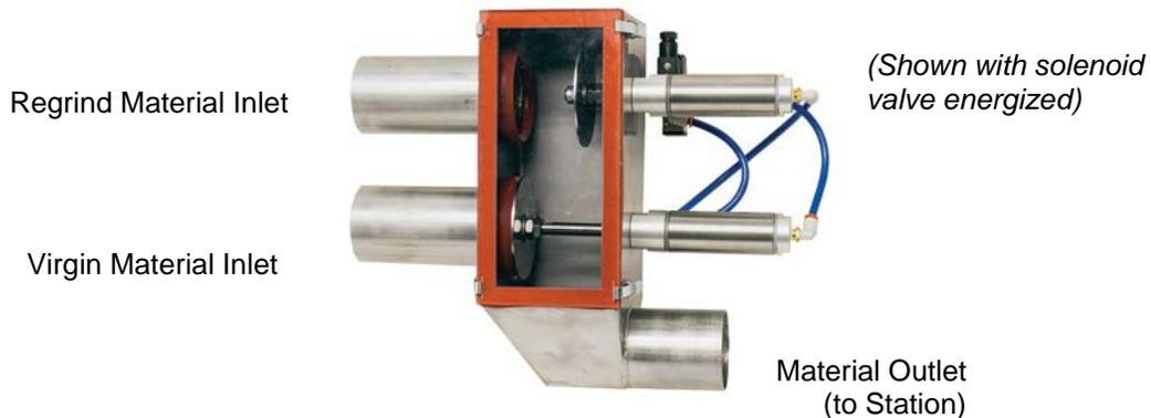
**NOTE:** The control energizes the proportioning valve's solenoid to pull regrind into the receiver station. When installing, please configure the valve's air piping to ensure the top port is closed to regrind in the de-energized state, and opens in the energized state. **IMPORTANT:** Premature gasket wear and failure may occur if the proportioning valve operates with the Regrind Material Inlet on the lower inlet port.
