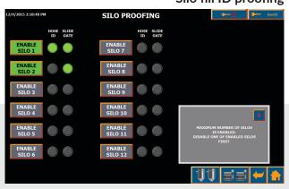
Truck unload ID proofing through FX2 control.
