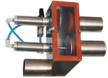
NOTE: The control energizes the proportioning valve's solenoid to pull regrind into the receiver station. When installing, please configure the valve's air piping to ensure the top port is closed to regrind in the de-energized state, and opens in the energized state. **IMPORTANT:** Premature gasket wear and failure may occur if the proportioning valve operates with the Regrind Material Inlet on the lower inlet port.
