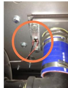
The MVP will continue in this mode until the elevated heat of the blower is reduced and the snap switch returns to its normal position, closing the vacuum breaker valve and allowing the vacuum system to operate normally. Note that during this temperature reduction mode, the conveying system connected to this pump is not operating, and material levels may run low, creating an alarm condition at the central control.
