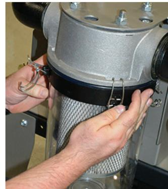
Release clamps to remove ClearVu cannister. Pull cannister straight down and empty any dust.
