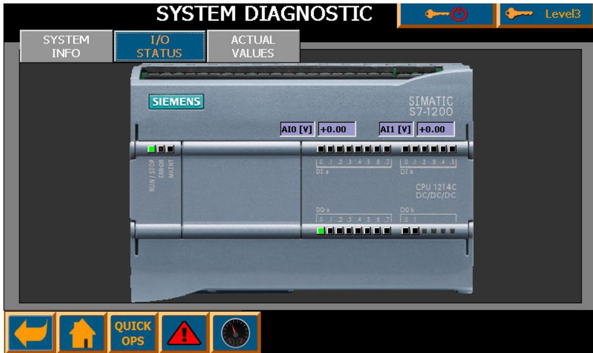
I/O Status view shows current LED status of PLC discrete inputs and outputs as well as current voltages read at analog inputs AI0 and AI1.
