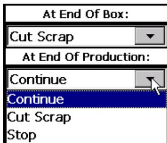
**At End of Box:** - (Requires box count to be enabled). Used to determine the action of the cutter when the part count has reached the end of box.
