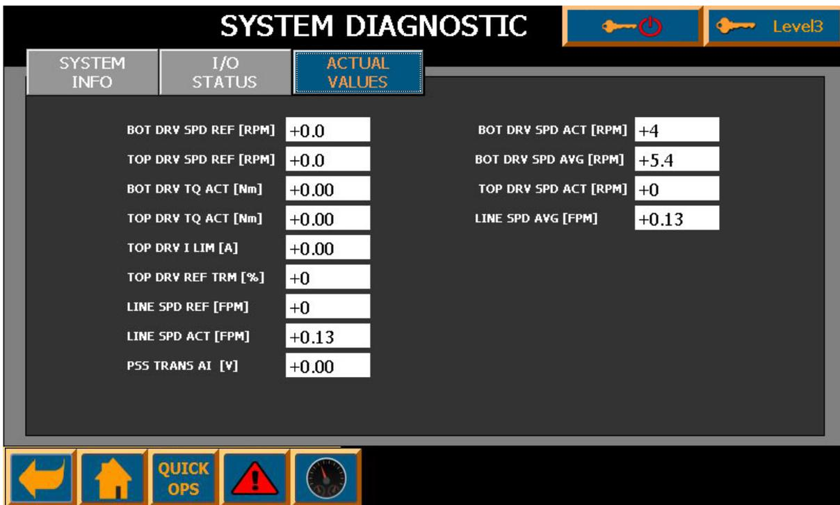
Actual Values view shows most actual machine values (e.g. motor speeds, torques etc.).
