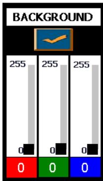
**Screen BACKGROUND Color** - Select the Red, Green and Blue content using the sliders or the numeric entry fields. The area around the check box will show the new background color. When the color is ok, press the checkbox to change the background colors of all the screens. Black(0,0,0) is the default background color. **Care should be taken to not use very bright colors or colors that match other fields because they will bleach out some items.**
