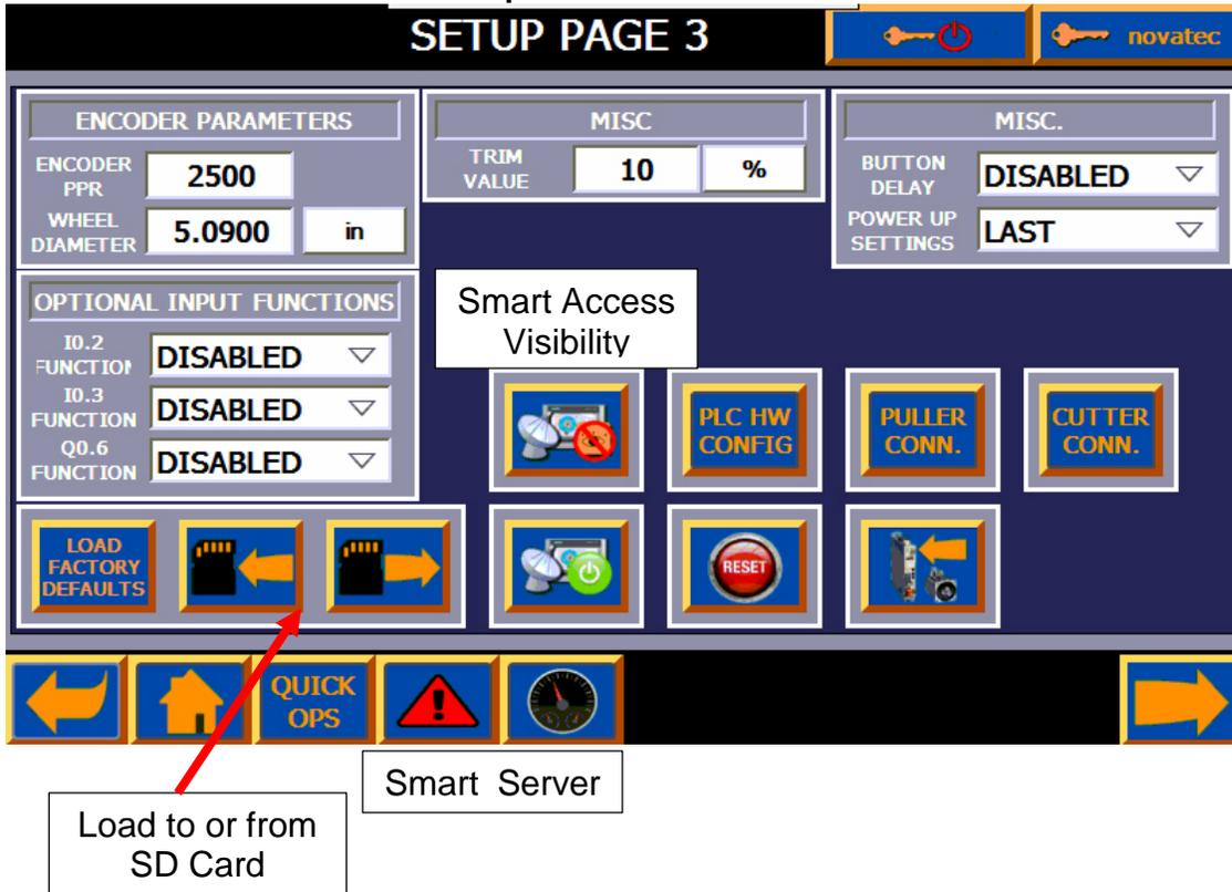
**ENCODER PARAMETERS** - ENCODER PPR (encoder pulse/rev.) WHEEL DIAMETER (encoder wheel diameter [in])
