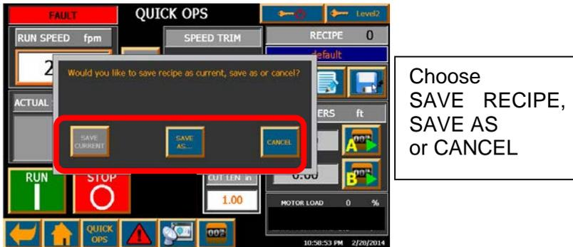
Click a recipe number and add ID and/or Name using alpha/numeric keyboard. Navigate through recipes with UP and DOWN arrows. Click to save.
