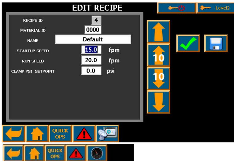
NOTE: A Default recipe is installed in each NOVATEC NPC Mini-Puller. It is intended as a default startup recipe for any production run. It can be changed.
