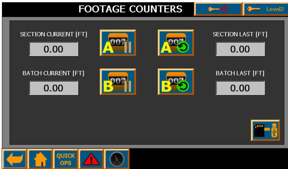
The footage counters start automatically when the NPC Mini-Puller is in the RUN mode.
