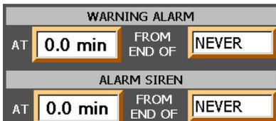
**Warnings and Alarms** - Signals can be set to activate a warning message or sound a siren when production reaches a certain point. The system calculates the time remaining at the current production rate and determines if the alarm should activate. Set the time in minutes and tenths of minutes and the event to activate the alarm which can be Never, End Of Box, End of
