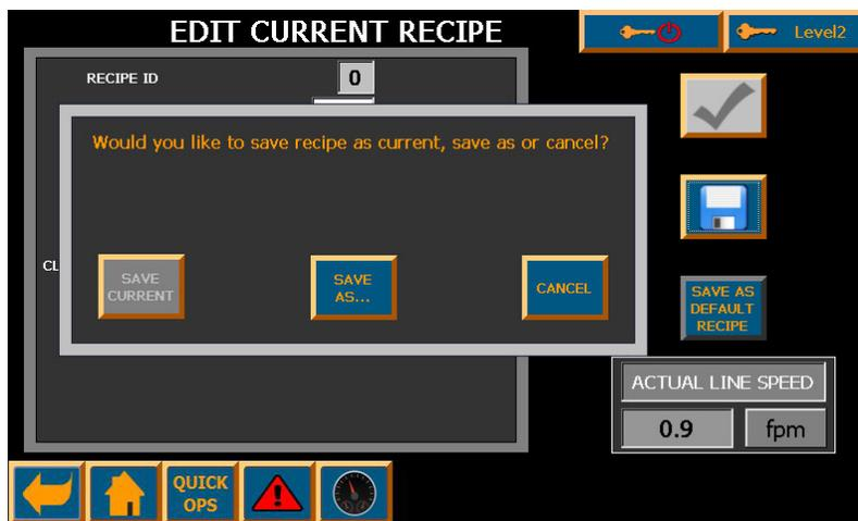
**NOTE:** Pressing SAVE also automatically activates changes made on the screen.
