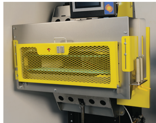
Fully enclosed belt guard show in locked position above and in open position below.
