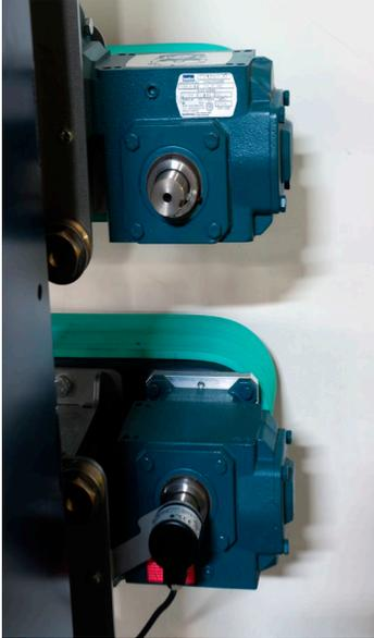
Double Reduction Helical Gear Reducer with optional external encoder mounted on the gear reducer for precise speed reading by other machinery (e.g. cutters).
