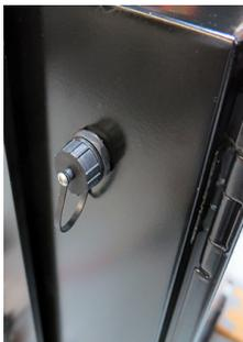
Industrial RJ-45 socket (shown with cap) for networking Puller PLC with Novatec Cutter or customer's plant PCs (data collection etc.).
