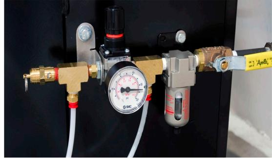
Belt tension bleed valve with pull ring
