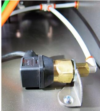
Alternately, the belt gap may be tensioned by looking down the belt gap from the upstream end of the traction assemblies. The gap will be convex if too loose and concave if too tight. The pressure switch will need to be readjusted if a pressure other than the factory set pressure for belt tension is set. Turn down pressure on regulator to desired setting. Remove machine air supply. Relieve pressure in traction assembly by pulling ring on pressure relief valve.
