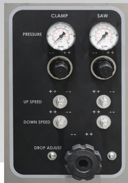
Pressure and speed control for saw blade and clamp motions
