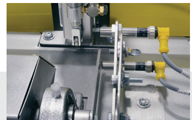
Easy table top access to blade stroke adjustment
