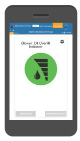
Oil overfill indicator warns if oil level is too high to prevent bearing and seal damage.
