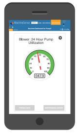
24-Hour pump utilization reflects duty cycle and potential expansion capacity.
