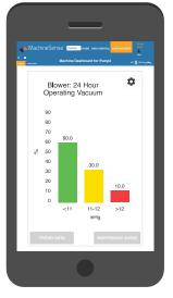
Operating vacuum patterns help diagnose pump and conveying operating health.
