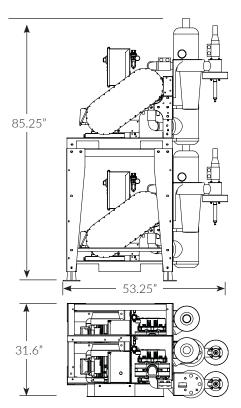
Above dimensions for 3 Hp or 5 Hp pumps stacked 2 - high. Add 2 inches to height for 10 Hp
