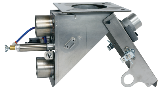
Hinged door opens for easy, complete clean-out when changing resin.
