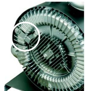
The VRB will continue in this mode until the elevated heat of the blower is reduced and the snap switch returns to its normal position, closing the vacuum breaker valve and allowing the vacuum system to operate normally. Note that during this temperature reduction mode, the conveying system connected to this pump is not operating, and material levels may run low, creating an alarm condition at the central control.
