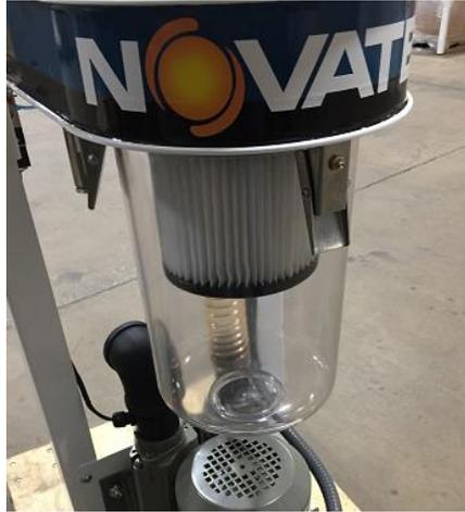
Figure 4: Filter element and bowl
