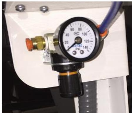
Figure 2: Vacuum valve air inlet
