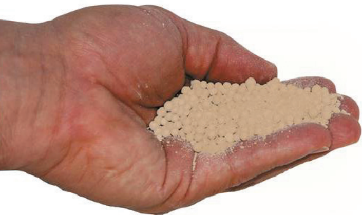
Worn or degraded desiccant beads cause higher energy costs.
