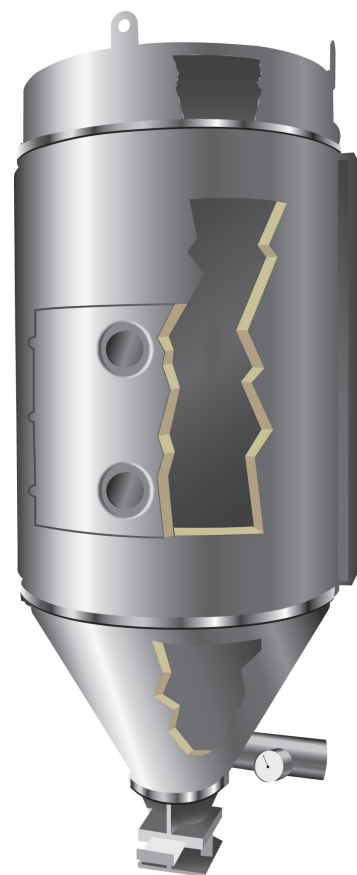
Hopper insulation should extend from bottom of cone to just below process return outlet.
