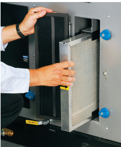
Drain plasticizer and wash filter regularly.
