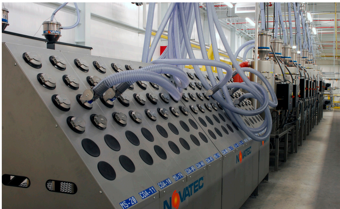
Auto ID validation of plastic pellets eliminates molding the wrong material.
