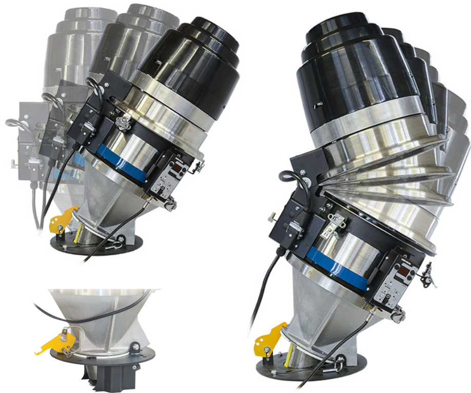
Loader pivots forward from operating position and a captive detent pin locks loader in place during operation. Lid pivots back and locks in place for easy access.
